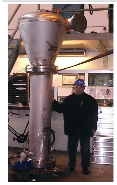
Figure 17 The 150-200 m 3 /h OptiMarin hydrocyclone installed on the C/S Regal Princess (Nilsen, private comm.)
