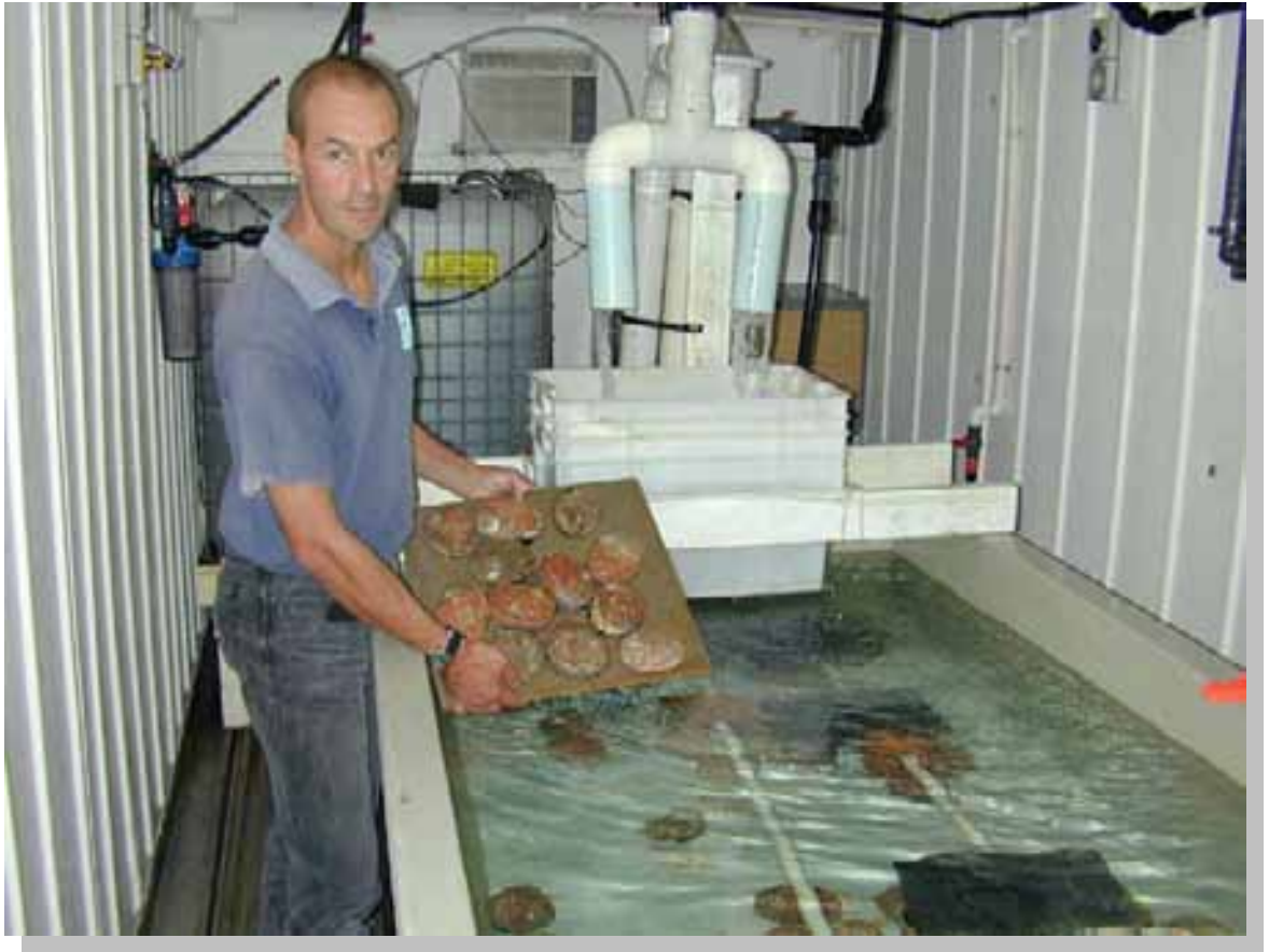
Figure 18 Controlled temperature reproductive conditioning system that employs recirculation and filtration of seawater to greatly reduce energy costs of heating or cooling (detailed specifications provided in Appendices 2 & 3 ).
