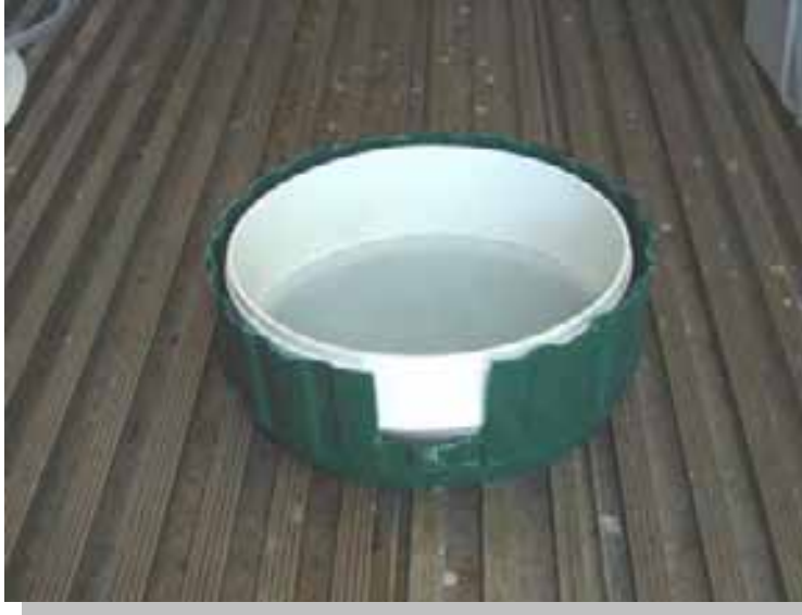
Figure 25 Screen and tub for wet harvesting and rinsing of eggs and larvae. N.B. Wall height of screen should be substantially greater than the depth of the tub to prevent loss of eggs or larvae through spillage or accidental overflow.
